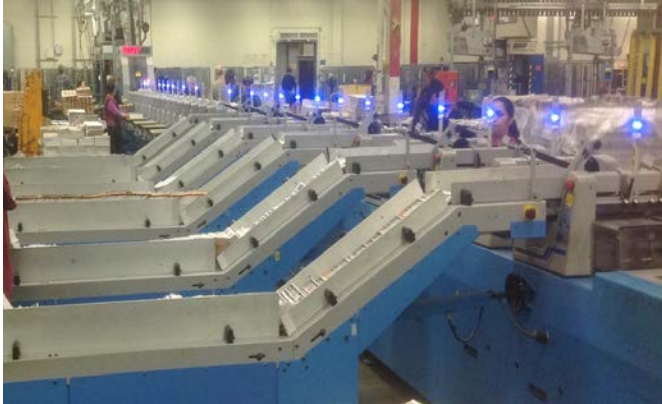
The Muller Martini SLS3000 inserter move from Pioneer Press to the Star Tribune also included a double drop and six hopper loaders.
