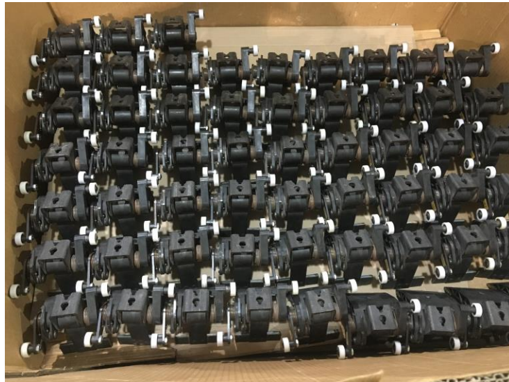
Grippers rebuilt and completed
