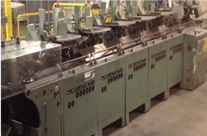
The Muller Martini 227 5:1 inserter was fully reconditioned, installed & commissioned by GIS, who also provided extensive operator training.
